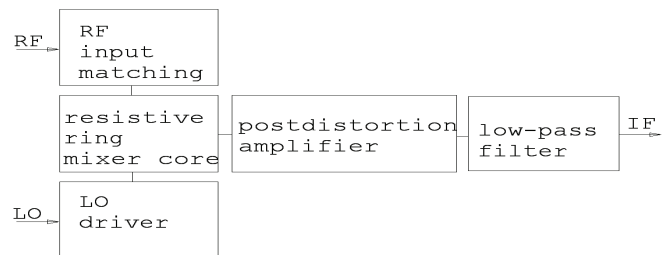
Figure 1. Block diagram of proposed high dynamic range mixer
