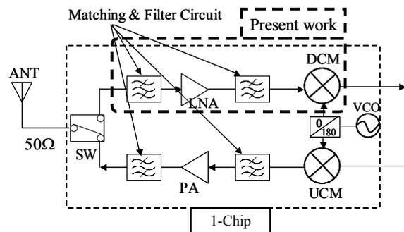
Fig. 1. Block diagram of single chip direct-conversion transceiver.
