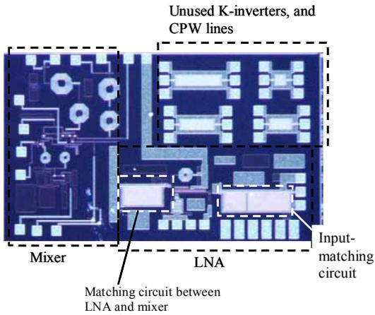
Fig. 4. Microphotograph of SiGe BiCMOS receiver front-end. (Chip size: 2mm x 3.5 mm)
