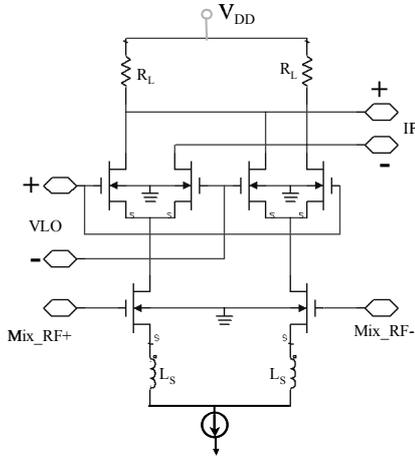
(b) Schematic of the designed DCM.
