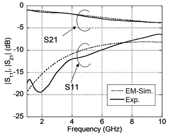
Fig. 7. Frequency responses of the CPW meanderline.
