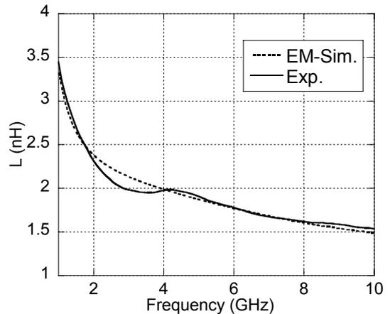
Fig. 8. Frequency dependence of the inductance ( $L$ ) of the  $K$ -inverter
