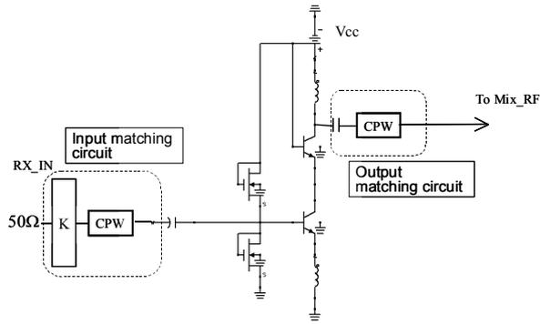
(a) Schematic of the designed LNA.
