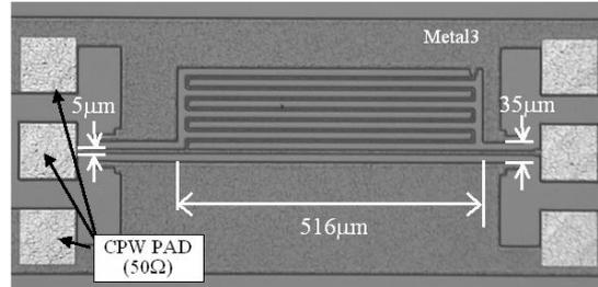
Fig. 6. Microphotograph of the  $K$ -inverter. (Taken out from another fabricated chip which is not shown in Fig. 4).
