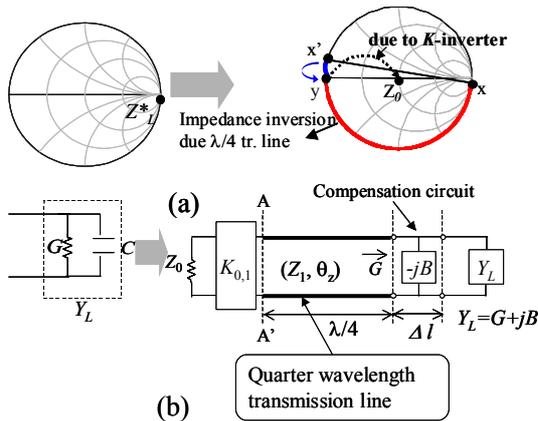
Fig. 3. Design and circuit model of impedance-matching circuit (a) Smith chart representation (b) circuit model using  $\lambda/4$  CPW line and  $K$ -inverter.
