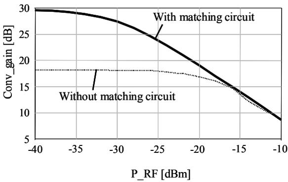
Fig. 5. Simulation results of the conversion gain of the mixer with and without the matching circuit between LNA and mixer.
