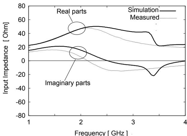
Fig. 9. Input impedance of the fabricated chip.
