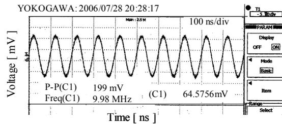
Fig. 14. Output of mixer sinusoidal waveform confirming the operation of the mixer measured by digital oscilloscope through a high-impedance probe (IF frequency = 10 MHz).
