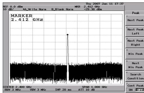
Fig. 15. An example of VCO output measured by spectrum analyzer.
