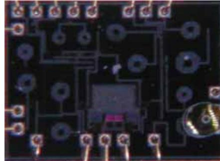
Fig. 13. Chip photo of proposed mixer connected with proposed VCO using CPW resonator. (Chip size = 1.3 mm x 1.7 mm including the matching circuits and biasing circuits at RF terminal).
