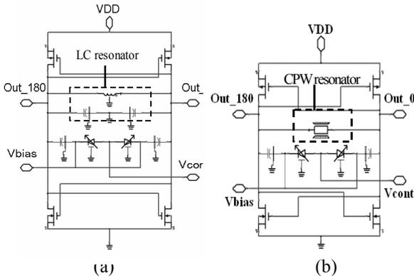
Fig. 7. Schematics of designed VCO using (a) LC resonator (b) proposed CPW resonator.
