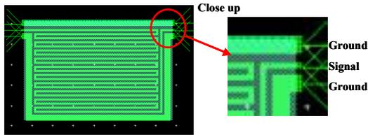
Fig. 6. Structure of CPW resonator on LSI process.
