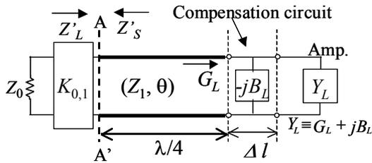
Fig. 3. Circuit model of the proposed matching circuit using  $\lambda/4$  transmission lines.
