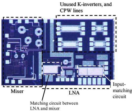
Fig. 11. Microphotograph of SiGe BiCMOS receiver front-end. (Chip size: 2mm x 3.5 mm)
