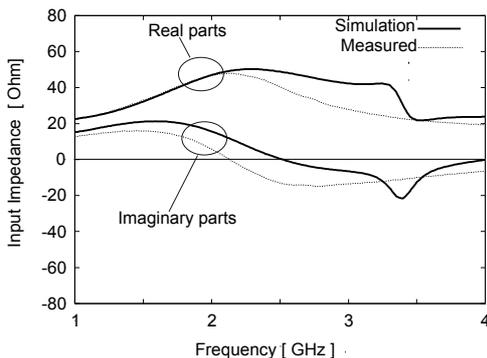
Fig. 12. Input impedance of the designed chip.
