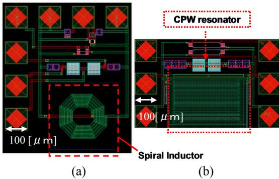
Fig. 8. Layout of the designed VCO using (a) LC resonator (b) proposed CPW resonator.
