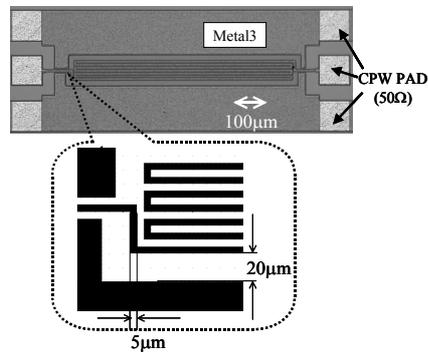
Fig. 9. Chip photo of conductor backed CPW.
