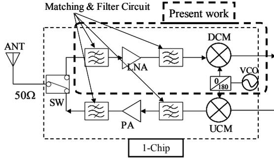
Fig. 1. Block diagram of direct conversion transceiver.
