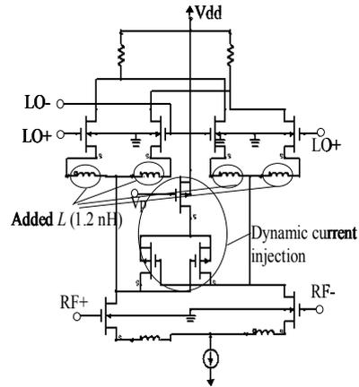
Fig. 4. Schematic of proposed double-balanced mixers using dynamic current injection method and four tuned inductors at switching stage transistors.
