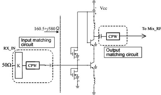
Fig. 2. Schematic of LNA with on-chip matching circuits.
