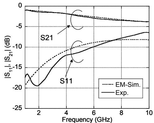
Fig. 10. Frequency responses of the CPW meanderline.
