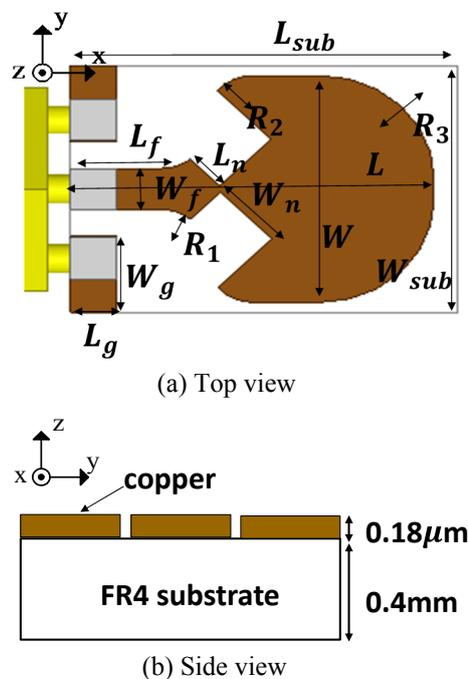
Figure 1. Design of the single antenna.
