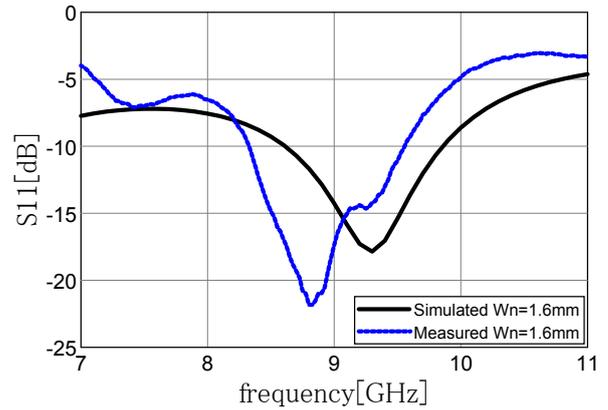
Figure 5. Measured and simulated return loss of the proposed antenna.
