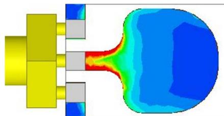
Figure 2. Simulation result of the current distribution without notches at 9.5GHz.
