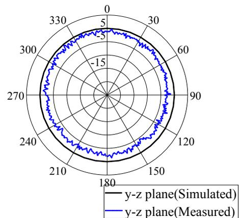
Figure 6. Measured and simulated radiation pattern of the proposed antenna.
