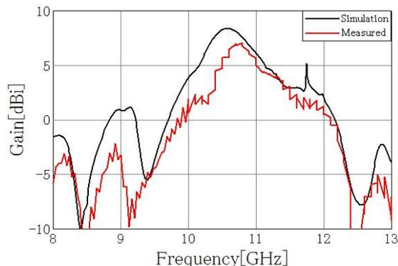
Figure 5. Measured and simulated antenna gains to the z-axis direction.
