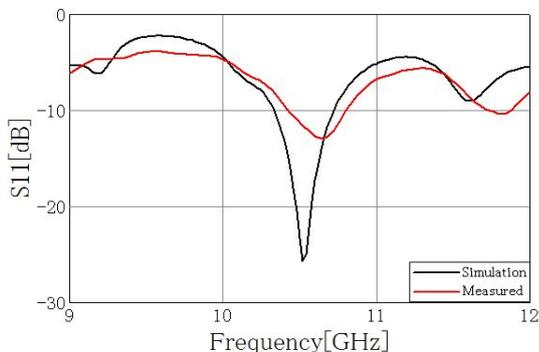
Figure 4. Measured and simulated return losses.
