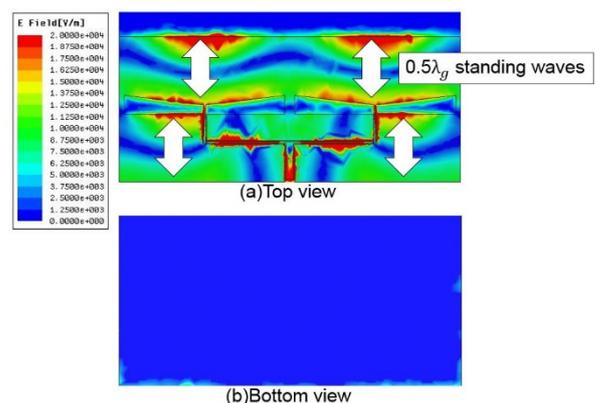
Figure 2. Top view (a) and bottom view (b) of the electric field of the 1 x 2 array antenna.
