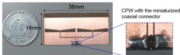
Figure 3. Photograph of proposed antenna.
