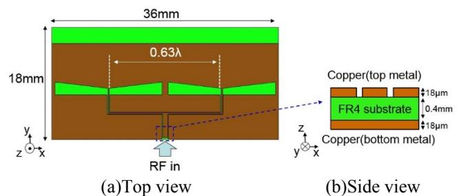
Figure 1. (a)Top and (b)side view of array antenna layout.
