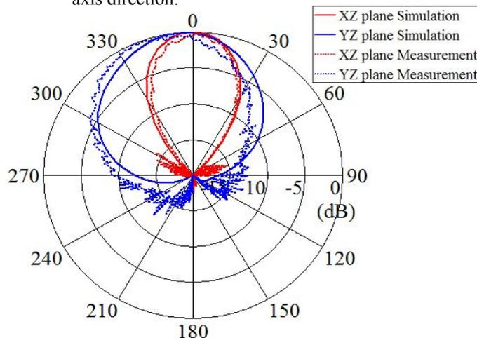
Figure 6. Measured and simulated radiation patterns.
