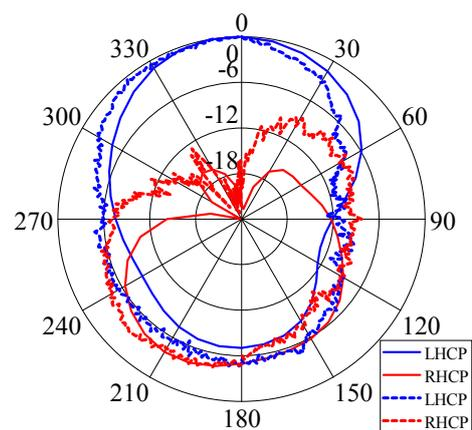
Fig. 6. Measured and simulated radiation of the proposed antenna.
