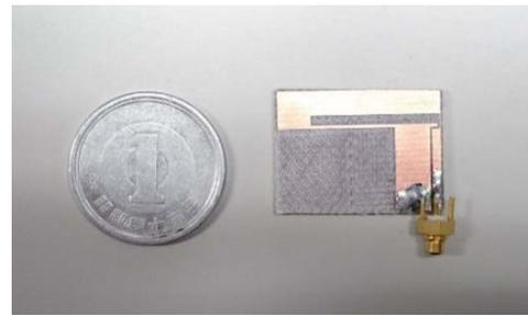
Fig. 3 Photograph of the proposed antenna.
