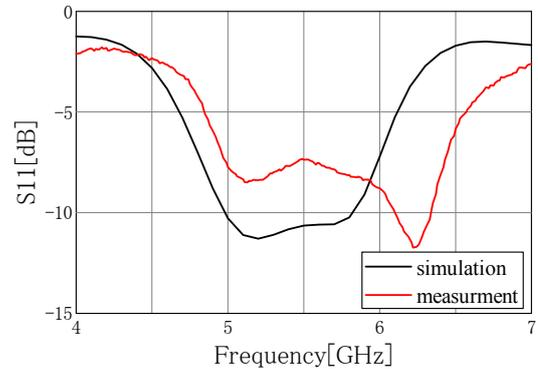
Fig. 4. Frequency responses of the measured and simulated reflection coefficient ( $S_{11}$ ).
