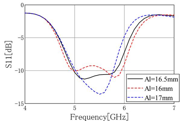
Fig. 2. Simulated  $S_{11}$  with different  $Al$ .
