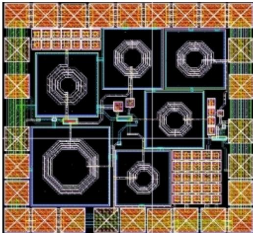
Figure 7. Layout of the proposed UWB PA on 0.18- $\mu\text{m}$  CMOS technology.
