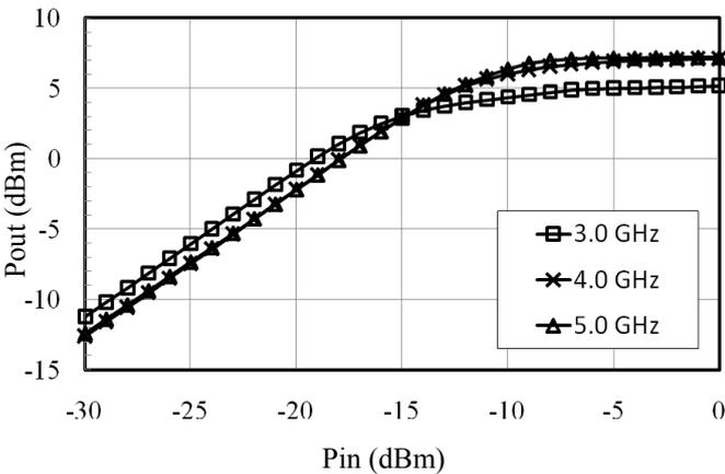
Figure 4. Simulated 1-dB compression point of UWB PA (post-layout).
