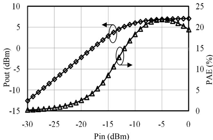
Figure 5. Simulated output power and PAE of UWB PA (post-layout).
