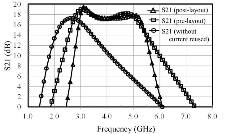
Figure 2. Simulated gain without current reused and with current reused (pre-layout and post-layout) of UWB PA.
