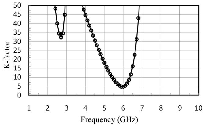
Figure 6. Simulated K-factor for stability of UWB PA (post-layout).
