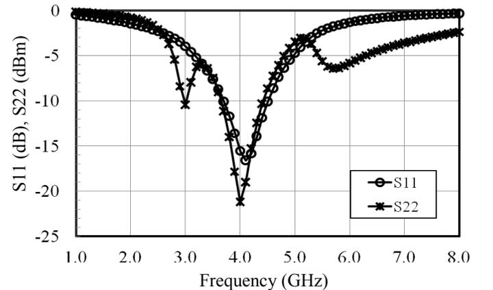
Figure 3. Simulated input and output return loss of UWB PA (post-layout).
