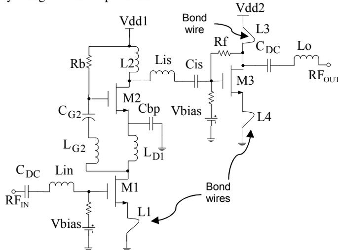
Figure 1. Schematic of the proposed current reused UWB PA.
