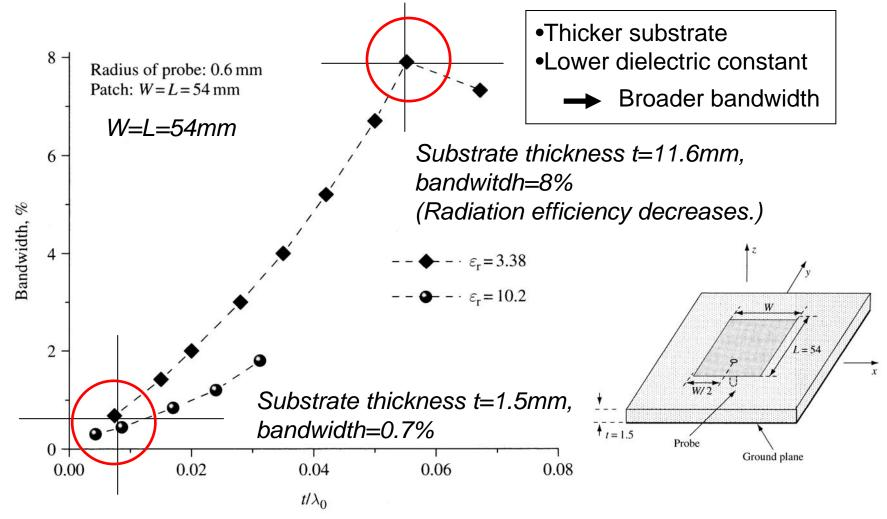
Figure 2.16 Bandwidth versus substrate thickness ratio.
