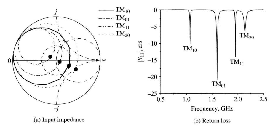
Figure 2.10 The input impedance and return loss  $|S_{11}|$ . W = 76mm, L = 54mm, t = 1.5mm,  $\varepsilon_r = 3.38$
