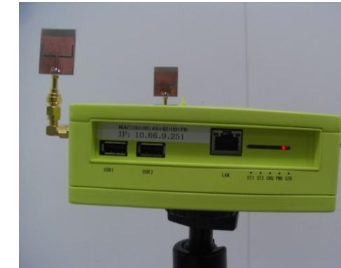
※ Speed: 36Mbps, Frequency: 52ch(5.26GHz), Amp. output: 17dBm(50mW)
